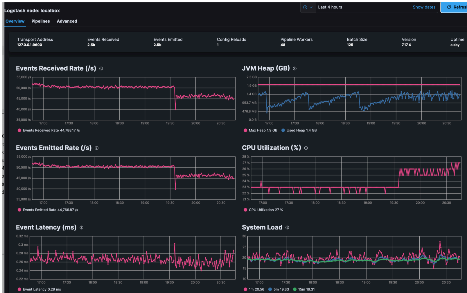
IMG011 - Logstash metrics with SUT pipeline batch size set at 500 (over previous 125, which is the default settings)
